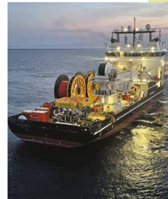
A vessel laying subsea cabling
